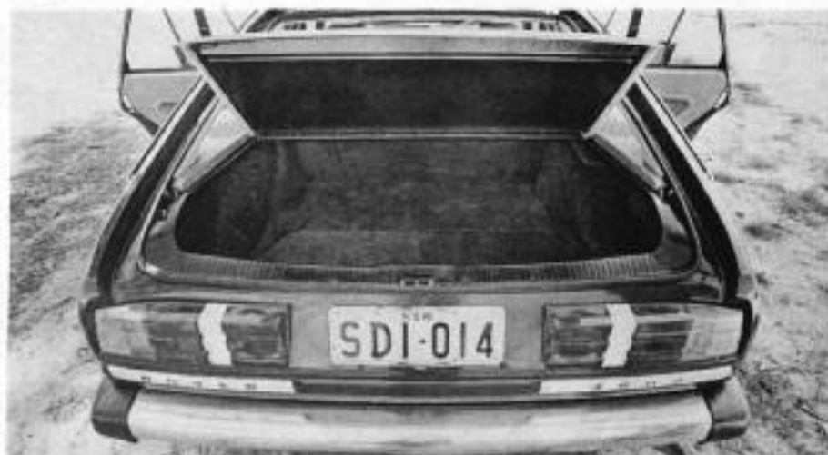
Conventional boot with parcel tray in place. Luggage sill is high. Rear window remains clean even in dirty weather, doesn't seem to need rear wiper/washer system.
